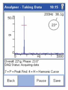
The FFT Analysis functionality of the Model 258B is a powerful and easy to use tool for measuring vibration signals, and breaking them down into their component frequencies.
