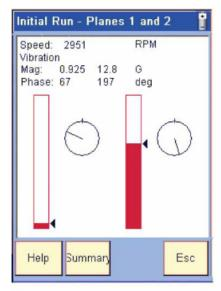
The Model 258B balancing module is a simple to use application allowing users to measure the unbalance in a rotating component and to calculate the required correction.
