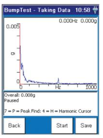
The Bump (Rap) Test module may be added to allow for the identification of the natural resonant frequencies of a mechanical structure. In some cases, the presence of a resonance can cause excessive levels of vibration and / or noise.
