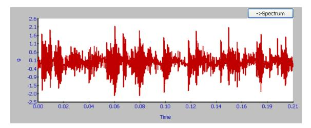
Figure 2 – vibration waveform from a damaged bearing
