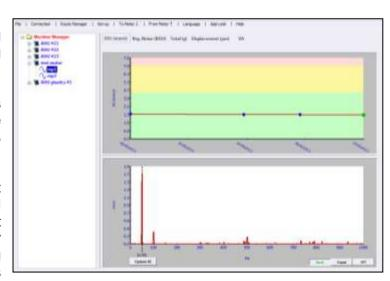
been selected from the menu tab at the top of the screen). The bottom half of the screen will show the frequency plot for the currently selected reading (identified by the green marker in the trend plot).
