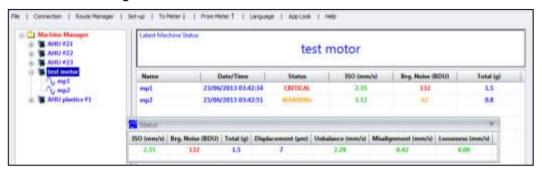
Clicking on any of the Vib Points will open up a window for that particular Vib Point and display all its readings graphically as shown below. Individual graphs of the various readings taken on the Vib point can be selected using the row of tabs displayed above the graphs.
