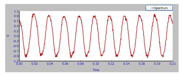
Figure 1 – vibration waveform from a good bearing
