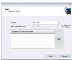
Each machine can be given a name (any length) and also a name to be used by the MachineryMate™ 800, which must be a maximum of 14 characters long.
