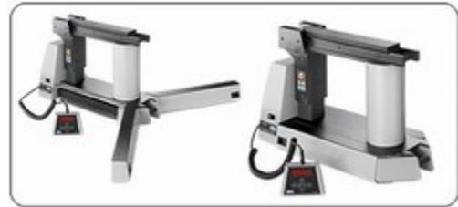
Maximum efficiency is achieved by placing the induction coil outside the heater's housing, in the centre of the bearing, resulting in shorter heating time and lower energy consumption. The LED operating display and control panel are integrated in a remote control, which makes the heater easy to use. To suit different operating voltages worldwide, the TIH 220m is available in different voltage variants.
