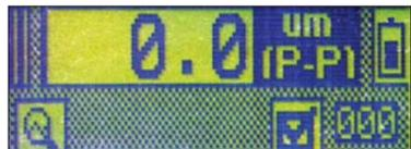
For those precision machines that have very low vibration levels, a precision reading is necessary. In addition to an extra quiet accelerometer that is supplied as a standard accessory, both vPod and vPod II incorporate a built-in gain circuit to amplify small vibration signals and show the reading in precision mode when you turn the gain mode on. This one button gain function allows the user to increase precision by one decimal place.
