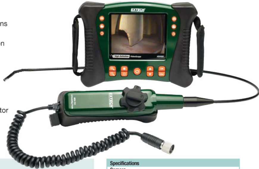
A. Articulating (6mm diameter) camera tip adjusts up to 320° viewing angle with four built-in bright LED lights illuminate dark areas B. HDV-WTX — Optional Wireless Transmitter transmits video to the main display from tight or hard to reach places up to 100ft (30m) away
