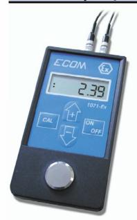
With the 1071-Ex measurements of wall thicknesses can be made quickly and accurately in the range of 0.03 to 15.7" (0.7 to 400 mm).
