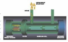
The filtered infrared energy passes through the sampling cell, striking the infrared detector. D-TEK Select is ready to sense any refrigerant.
