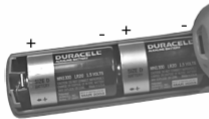
Figure 1. Properly Installed Alkaline Batteries
