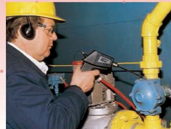
Ultraprobe 100 testing pump valve leaks
