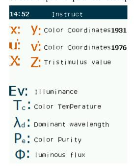
The definition of photometric and colorimetric symbols are provided in the page for operation.
