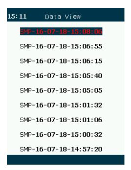
Data list is sorted by time, and device only stores latest nine dada. New data would cover previous data automatically.
