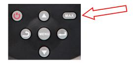
Every data will be stored into SD card under "MAX" measuring condition. Measuring screen is showed as followed:
