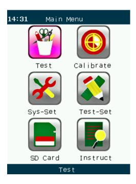
When we press the 'ok' key, it jumps into testing menu. User can check for color difference value, chromaticity diagram and RGB value.
