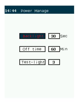
There are functions include screen backlighting time setting, auto-shut off time setting and backlight brightness adjustment.
