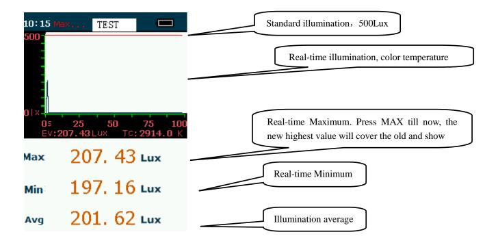
Under the "MAX" condition, Press the 'HOLD' key, the device stop measuring and keep the screen still, then give the tips about the appearing time of Maximum and Minimum value. See as followed:
