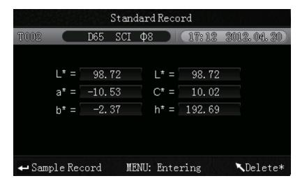
Here you can navigate between the different readings by using the arrow keys ( ↑ and ↓ ).
