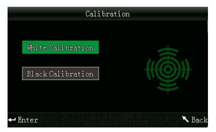
Here you can select between white and black calibration. Use the arrow keys ( ↑ and ↓ ) to make a selection and press Enter ← to confirm. A confirmation screen with instructions will appear.
