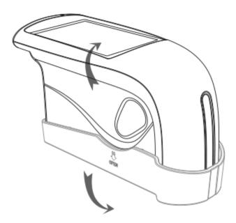
Figure 2 Separation Method
