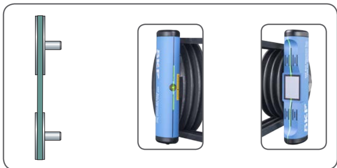
Figure 9: Pulleys perfectly aligned
